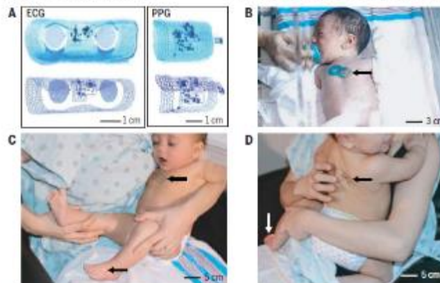
Wireless, skin-like systems for vital signs monitoring in neonatal intensive care. (A) Images and finite element modeling results for ECG and PPG devices bent around glass cylinders. (B) A neonate with an ECG device on the chest. (C and D) A mother holding her infant with a PPG device on the foot and an ECG device on the chest (C) and on the back (D).
